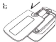
4.2.1 To press the battery cover groove, slip outward and open the battery cover;
