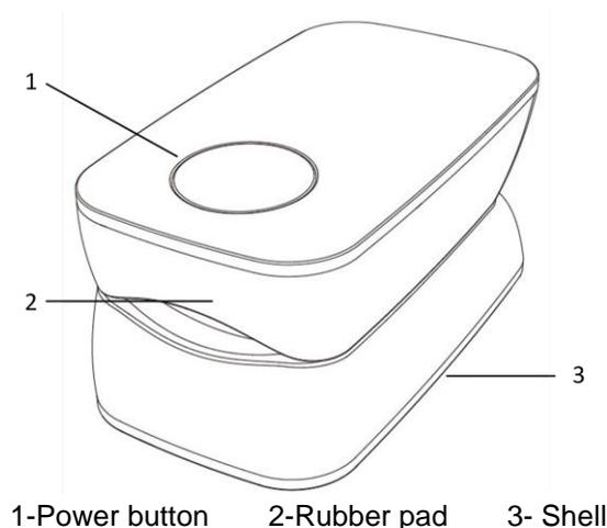
Diagram 1. Measurement hardware structure
